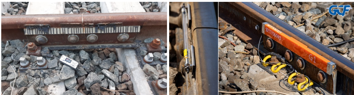
Figure 5. Left: electromechanical IRJ found detached along a railway line (photo A. Bracciali). Right: optical IRJ sensor (from [6]).
